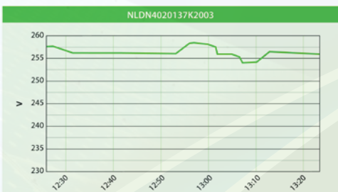
Graph below shows same day inverter output voltage consistently above 250V
