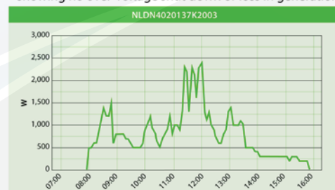
Graph below shows the same Omnik 3kWp inverter after Solar PV+ technology has been installed in Jan 2014. Clearly showing no over-voltage shut down or loss in generation
