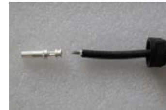
▲ Figure 4.7 Insert the Wire into the Connector Cap nut and contact pin
