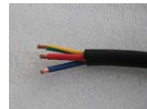
▲ Figure 4.13 Stripped AC Wires
