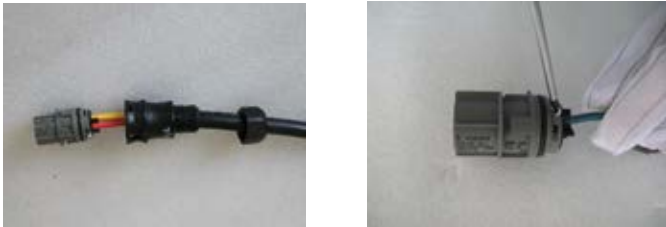
▲ Figure 4.14 Connect Wires to the Terminal
