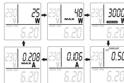
The MAX values can be cleared in the relevant display by pressing the „SET“ key (8) for approx. 3s. A short beep confirms the deletion process.
