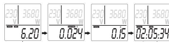
The total operating time can be deleted in the displayed function "TOTAL TIME". To do this, set the display on the top right (6) to "A" and press the key "SET" (8) and hold it for approx. 3 seconds. A short beep will confirm the deletion process.
