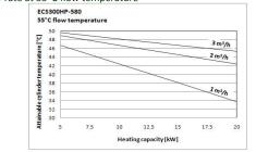
Attainable cylinder temperature as a function of heat pump output, flow rate at 65°C flow temperature
